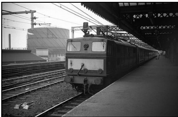
Sheffield Victoria station 5th June 1968. EM1 E26055, named Mentor and in green livery, prior to my departure for Manchester Picadilly and a visit to Patricroft shed. Thirteen EM1s, including the original LNER 26000, were fitted with boilers for heating passenger stock. The remaining non-boiler fitted EM1s were confined to freight workings.
