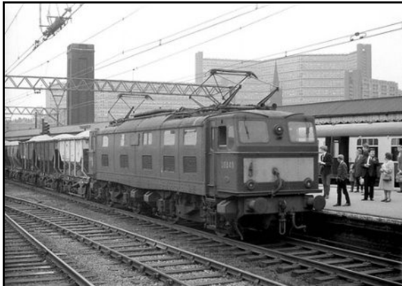
Sheffield Victoria station Spring 1969. EM1 E26049 1500v dc electric on a north bound freight.
