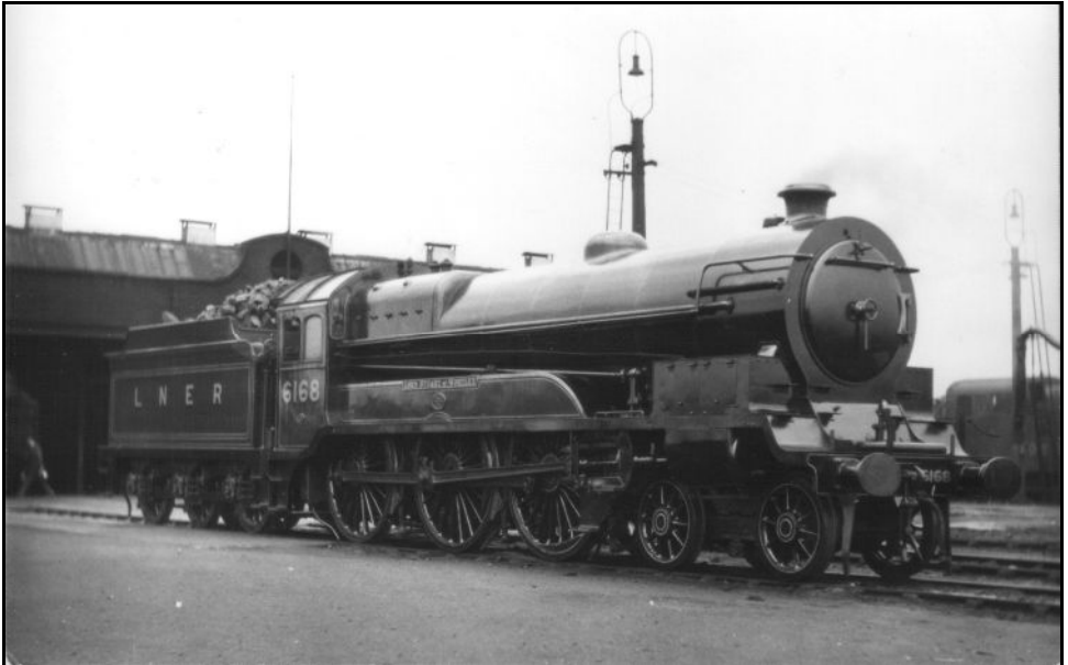
LNER class B3/2 4-6-0 no.6168 Lord Stuart of Wortley with side-window cab.
