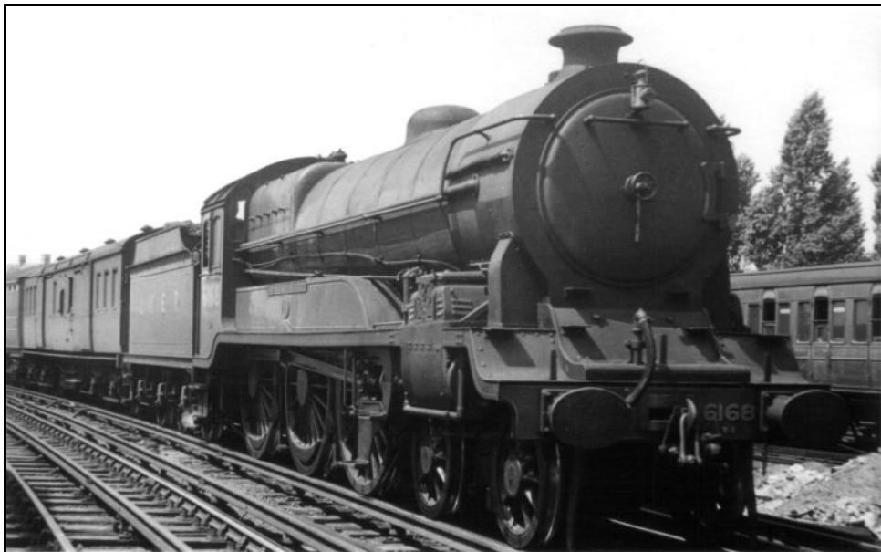
LNER class B3/2 4-6-0 no.6168 Lord Stuart of Wortley passing Harrow in 1938 with casing over Caprotti valve gear removed. photo : C.R.L.Coles
