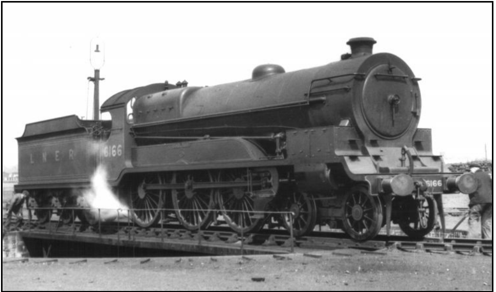
LNER class B3/2 4-6-0 no.6166 Earl Haig with cut-away cab.
